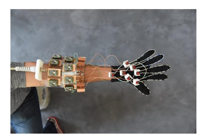
In a first for MRI, a glove-shaped detector proved capable of capturing images of moving fingers. The technology showed how tissue types moved in concert, which could be useful in cataloging differences seen in injury. Credit: NYU School of Medicine
