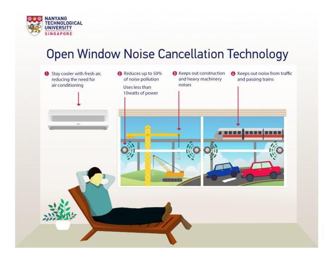
Infographics showing how the noise cancellation device developed by NTU
