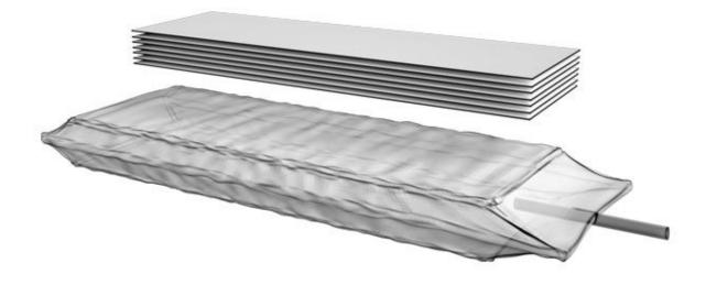
The structure consists of multiple layers of flexible material wrapped in a plastic envelope and connected to a vacuum source. Credit: Yashraj Narang/Harvard SEAS
