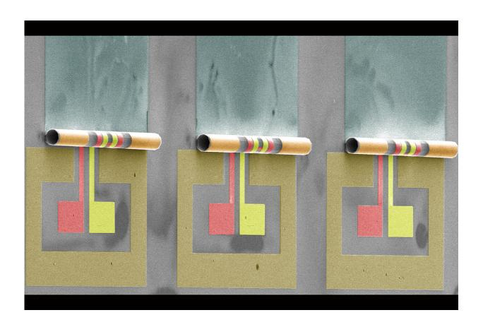
Illinois engineers roll toward smaller, more efficient radio frequency transformers that take 10 to 100 times less space on a microchip. Credit: Wen Huang
