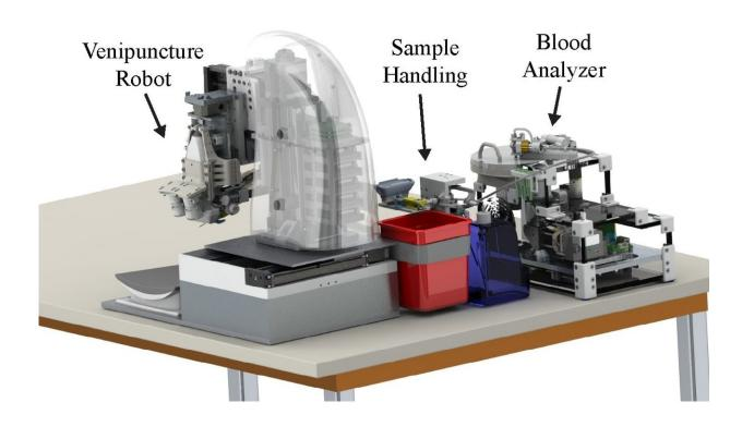
This fully automated device includes an image-guided robot for drawing blood from veins, a sample-handling module and a centrifuge-based blood analyzer. Credit: Max Balter
