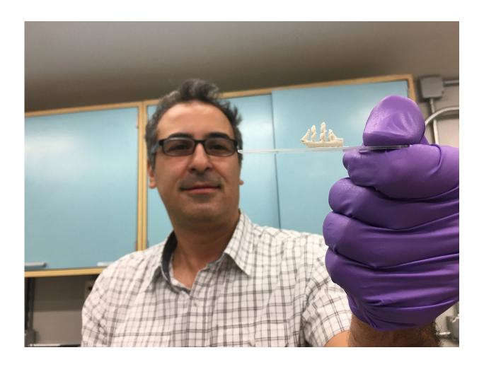
A new 3-D printing technique allows materials with the consistency of clay or cookie dough to be used to manufacture a variety of shapes. Purdue Univeristy assistant professor Emre Gunduz used ultrasonic vibrations to maintain a flow of the material through the printer nozzle. Credit: Purdue University photo/Jared Pike
