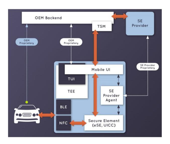
The diagram provides a high level architecture highlighting the focus of CCC efforts including the interfaces to be standardized. Credit: Car Connectivity Consortium
