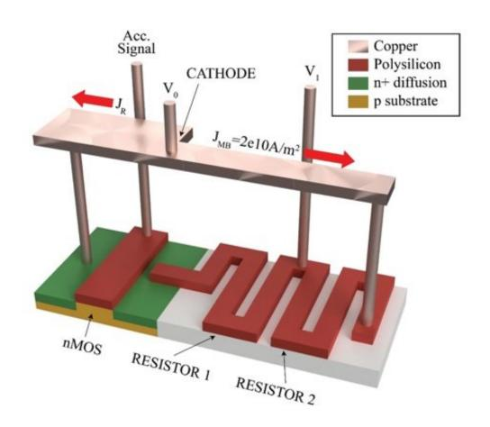
A configurable reservoir-based fast electromigration aging design for interconnects. Credit: Sheldon Tan
