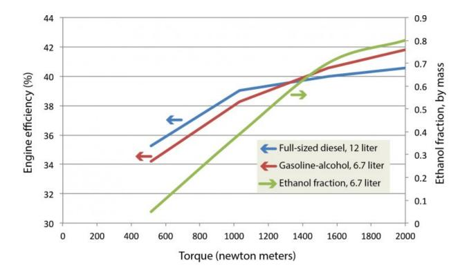
This figure shows engine efficiency at various levels of torque (rotational force)
