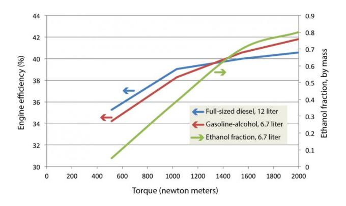
This figure shows engine efficiency at various levels of torque (rotational force)
