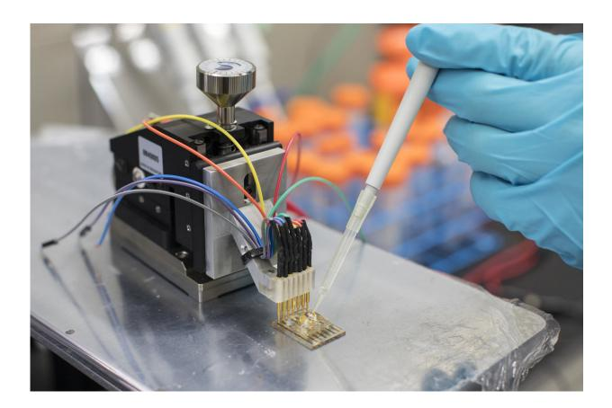
A low-cost sensor made from semiconducting plastic could be used to diagnose or monitor a wide range of health conditions, such as surgical complications or neurodegenerative diseases. Credit: KAUST
