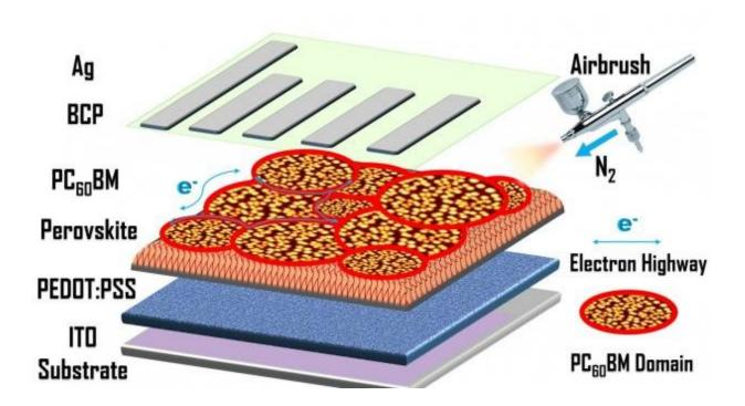
A model of a perovskite solar cell, showing its different layers. Professor André D. Taylor has been working to solve fabrication challenges with perovskite cells. Credit: Royal Society of Chemistry, *Nanoscale* (2018). DOI: 10.1039/C8NR01763H
