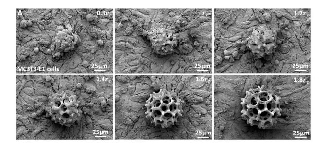
Microrobots of different sizes were found to have different cell-carrying capacities. Credit: Li et al., *Sci. Robot.* 3, eaat8829 (2018)
