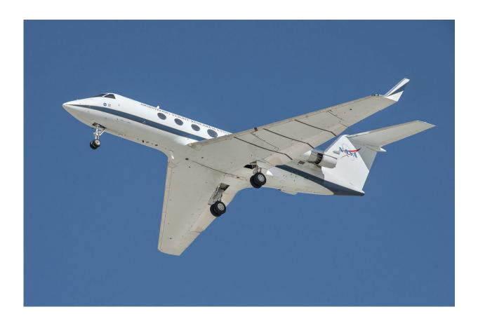
The ARM flights were flown on NASA's SubsoniC Research Aircraft Testbed G-III aircraft, or SCRAT, at NASA's Armstrong Flight Research Center in California. NASA combined three technologies, including Landing Gear Noise Reduction, landing gear cavity treatments, and the Adaptive Compliant Trailing Edge flexible wing flap, to demonstrate a reduction in airframe noise in excess of 70 percent. This may reduce aircraft noise for communities that live near airports. Credit: NASA/Ken Ulbrich
