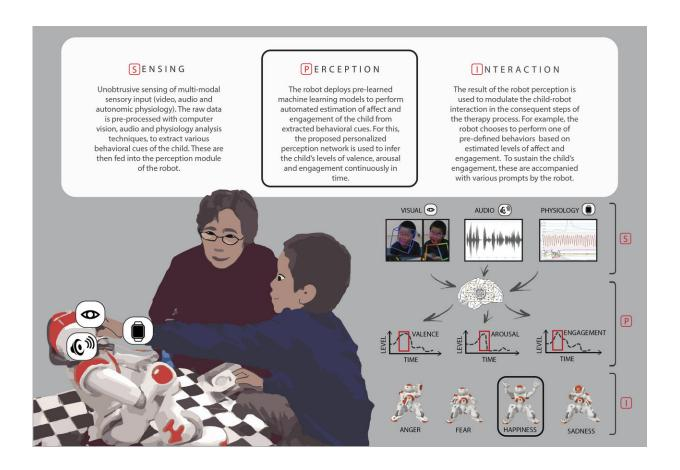
Overview of the key stages (sensing, perception, and interaction) during robot-assisted autism therapy. Credit: Rudovic et al., *Sci. Robot.* 3, eaao6760 (2018)
