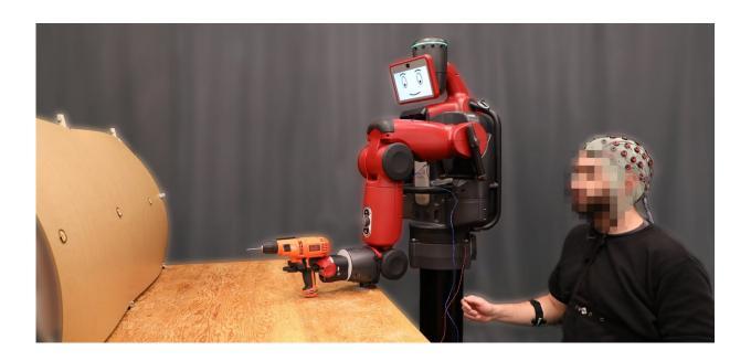
By monitoring brain activity, the system can detect in real time if a person notices an error as a robot does a task. Credit: MIT CSAIL
