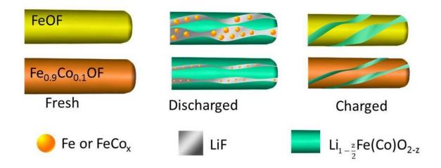
Substituting the cathode material with oxygen and cobalt prevents lithium from breaking chemical bonds and preserves the material's structure. Credit: Brookhaven National Laboratory
