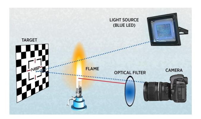
Graphic illustrating the NIST narrow-spectrum illumination method for imaging through fire. Blue LED light is directed through a gas fire, reflects off the target object behind the flames and is captured by a camera after passing through an optical filter. This reduces the observed intensity of the flame by 10,000-fold and yields highly detailed images. Credit: Graphic created by N. Hanacek/NIST based on a concept by M. Hoehler/NIST
