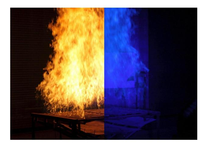
To improve the ability of researchers to "see" through fire, NIST has developed an imaging system using ordinary blue light to dramatically clear the picture. Credit: National Fire Research Laboratory/NIST
