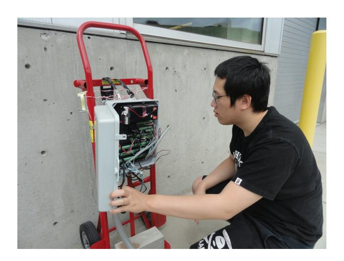
Chemical engineering student Ka Fung Wong looks at the data log, which is used to gather data from sensors buried under the concrete test plot. Credit: WSU
