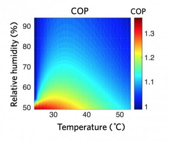
This chart shows the coefficient of performance (COP) of the membrane-based cooling system with vacuum pump at various combinations of ambient temperature and humidity. Credit: Massachusetts Institute of Technology
