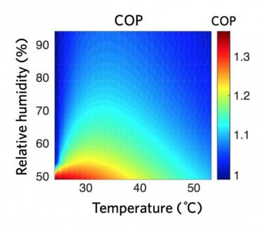
This chart shows the coefficient of performance (COP) of the membrane-based cooling system with vacuum pump at various combinations of ambient temperature and humidity. Credit: Massachusetts Institute of Technology
