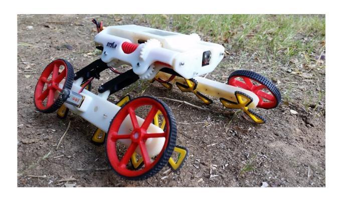
Ben-Gurion University of the Negev researchers designed the Rising Sprawl-Tuned Autonomous Robot (RSTAR) to function simply and reliably, change shape and overcome common obstacles without any external mechanical intervention. RSTAR uses adjustable sprawling legs angled downwards and outwards from its body to creep and crawl and climb over and through a variety of obstacles and surfaces. Credit: Ben-Gurion U
