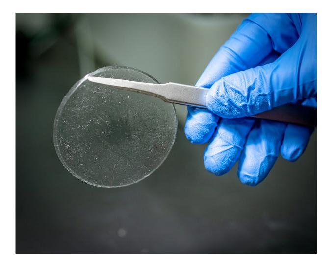
A sodium-ion conducting membrane for a nonaqueous redox flow battery. Credit: ORNL/Carlos Jones
