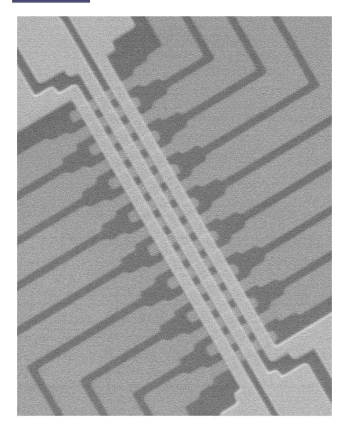
Electron microscope image of the memristor array. Credit: Yeonjoo Jeong, Nanoelectronics group, University of Michigan.
