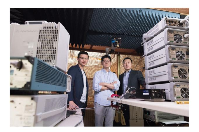
Georgia Tech researchers are shown with electronics equipment and antenna setup used to measure far-field radiated output signal from millimeter wave transmitters. Shown are Graduate Research Assistant Huy Thong Nguyen, Graduate Research Assistant Sensen Li, and Assistant Professor Hua Wang. Credit: Allison Carter, Georgia Tech
