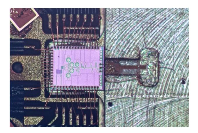
The clock transmitter chip (pink) wired to a circuit board package. Connected is a metal gas cell (right), in which a 231.061 GHz signal generated from the chip excites the rotation of carbonyl sulfide molecules. Because the peak rotation of the molecules is constant, it can be used as a reference point to keep accurate time. Credit: Massachusetts Institute of Technology
