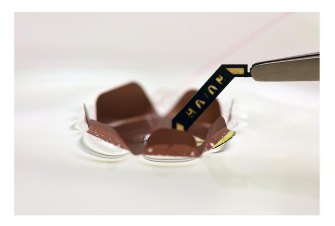
HAMR's multifunctional foot pads rely on surface tension and surface tension induced buoyancy when HAMR needs to swim but can also apply a voltage to break the water surface when HAMR needs to sink. Credit: Yufeng Chen, Neel Doshi, and Benjamin Goldberg/Harvard University
