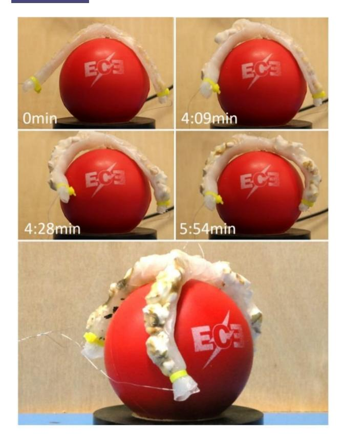
Fiber-reinforced elastomer actuator powered using popcorn wrapped in
