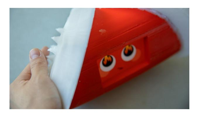
The robot prototype expresses its "anger" with both its eyes and its skin, which turns spiky through fluidic actuators that are inflated under its skin, based on its "mood.". Credit: Lindsay France
