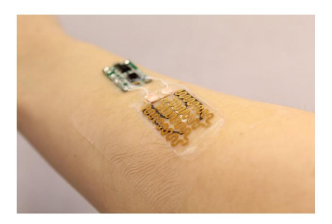
A smart bandage placed on an arm. Temperature and pH sensors in the bandage (right) are read by a microprocessor (left), which may trigger release of drug from the bandage by sending a current through heating elements. Credit: Tufts University
