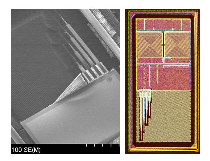
These figures show pre- and post-fabricated wireless neural probes chip micrograph. Purdue University researchers developed an electronic chip that can read signals from several nerve endings and wirelessly transmit them without needing a battery or any other off-chip component. Credit: Purdue University
