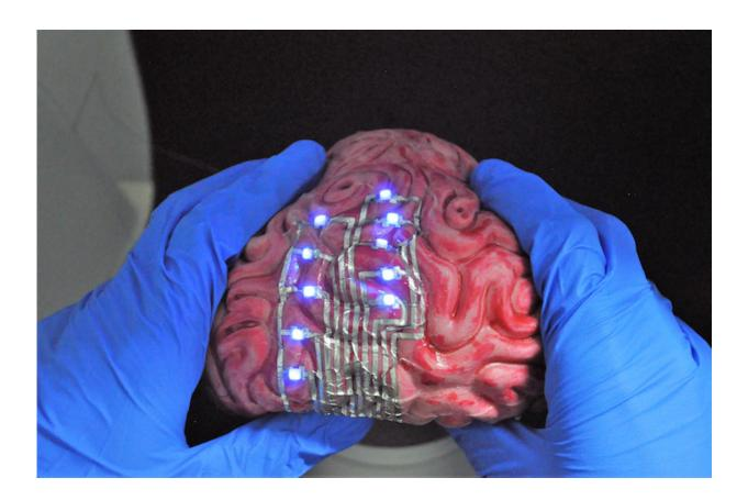
These stretchable, inexpensive, tattoo-like circuits can conform and adhere to highly curved 3D surfaces like a model of a human brain. Credit: College of Engineering, Carnegie Mellon University
