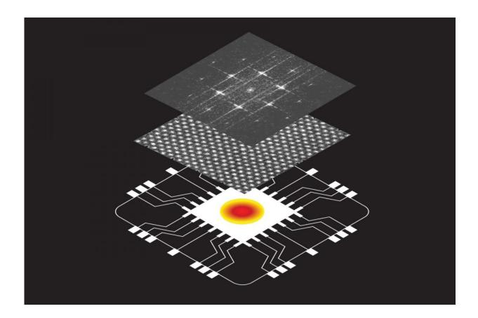
Illustration showing a schematic of a computer chip with a hotspot (bottom); an electron microscope image of defect-free boron arsenide (middle); and an image showing electron diffraction patterns in boron arsenide. Credit: Hu Research Lab / UCLA Samueli
