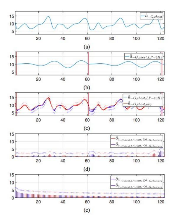
Illustration of the binary key generation block. (a) Gait signal ^a–G,chest (m/s2). (b) ^a–G,chest (m/s2) filtered by the 3 Hz low-pass filter. (c) Bit extraction by comparing a^–G,chest filtered by the 10 Hz low pass filter and the averaged a^–G,chest. (d) Energy difference, δ, between ^a–G,chest,LP=10Hz and ^a–G,chest,avg (e) Re-indexed binary keys using the associated reliability vectors. Credit: Sun & Lo
