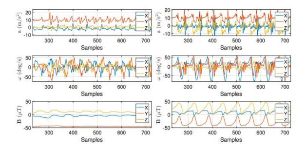
IMU outputs at the chest and shin positions, a=acceleration,  $\omega$ =angular velocity, and B=magnetic field. Credit: Sun & Lo
