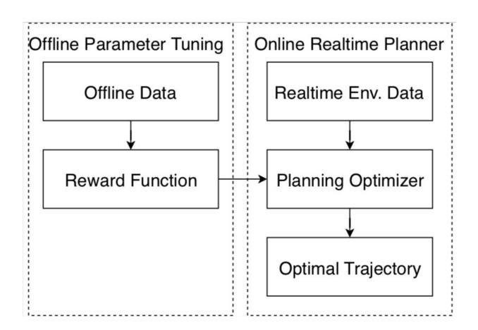
Data-driven autonomous driving motion planner on the Apollo platform. Credit: Fan et al.
