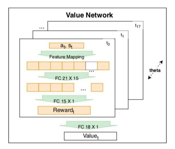
The value network inside the siamese model is used to capture driving behavior based on encoded features. The network is a trainable linear combination of encoded rewards at different times t = t0,...,t17. The weight of the encoded reward is a learnable time decay factor. The encoded reward includes an input
