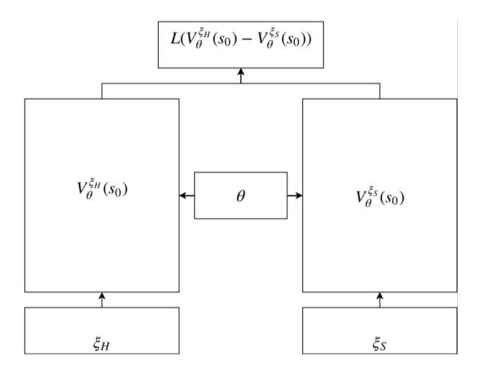
Siamese network in RC-IRL. The value networks of both the human and the sampled trajectories share the same network parameter settings. The loss function evaluates the difference between the sampled data and the generated trajectory via the value network outputs. Credit: Fan et al.
