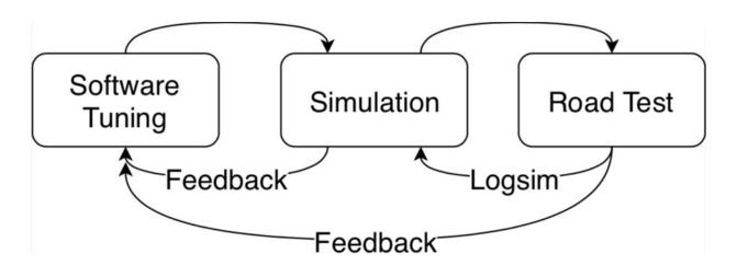
Algorithm tuning loop for the motion planner in the Apollo autonomous driving platform. Credit: Fan et al.
