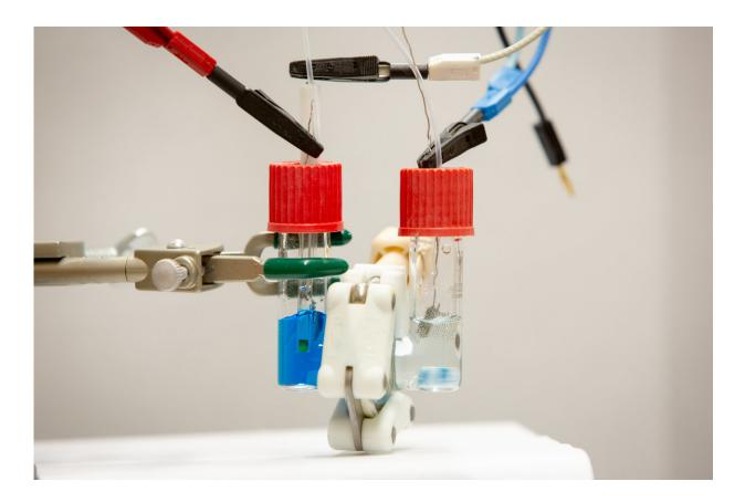
A simple liquid-based battery containing a methylene blue solution (left side), and a colorless solution of leuco methylene blue (right), which is methylene blue with added electrons. Credit: Meredith Forrest Kulwicki/University at Buffalo
