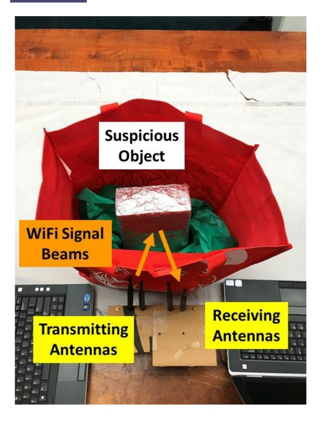
Using common WiFi, this low-cost suspicious object detection system can detect weapons, bombs and explosive chemicals in bags, backpacks and luggage.
