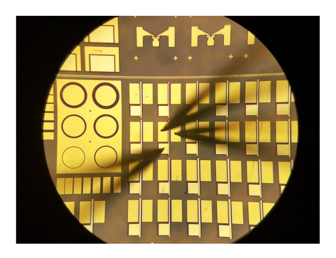
Credit: University at Buffalo An optical microscope image of an array of the transistor. The three dark arrows are the needle probes contacting the terminals of the transistor for electrical measurement. Credit: Ke Zeng, University at Buffalo
