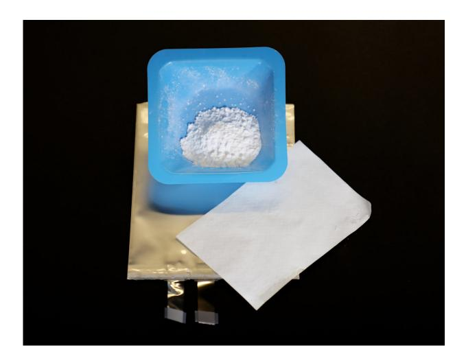
Adding powdered silica (in blue container) to the polymer layer (white sheet) that separates electrodes inside a test battery (gold bag) will prevent lithium-ion battery fires. Credit: Gabriel Veith
