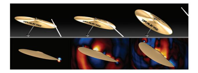
By computing pressure waves cast off by rapidly moving and vibrating surfaces – such as a cymbal – a new sound synthesis system developed by Stanford researchers can automatically render realistic sound for computer animations. Credit: Timothy Langlois, Doug L. James, Ante Qu and Jui-Hsien Wang
