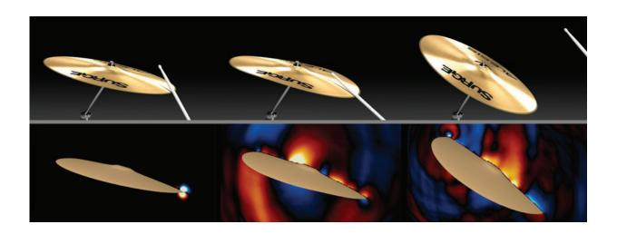
By computing pressure waves cast off by rapidly moving and vibrating surfaces – such as a cymbal – a new sound synthesis system developed by Stanford researchers can automatically render realistic sound for computer animations. Credit: Timothy Langlois, Doug L. James, Ante Qu and Jui-Hsien Wang
