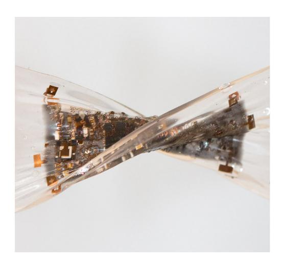
This '3-D stretchable electronic' device can stretch, bend and twist without compromising electronic function. Credit: Zhenlong Huang
