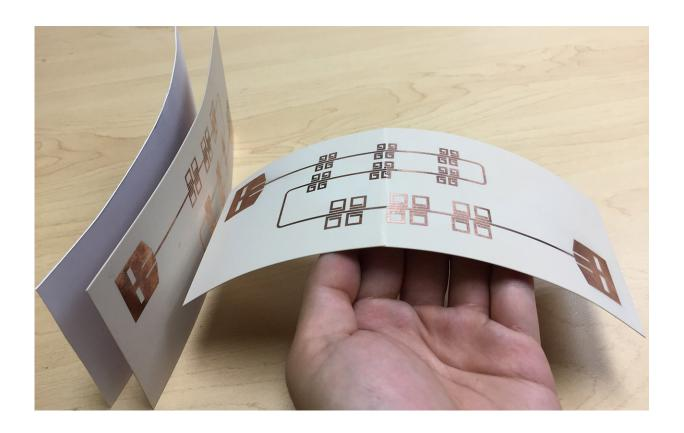
Printed thin, flexible LiveTag tags in comparison with a piece of photo paper (far left). Credit: Xinyu Zhang *et al*.
