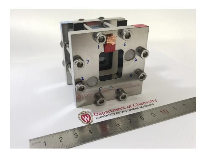
The scale of a new integrated solar flow battery. Credit: Wenjie Li, UW-Madison
