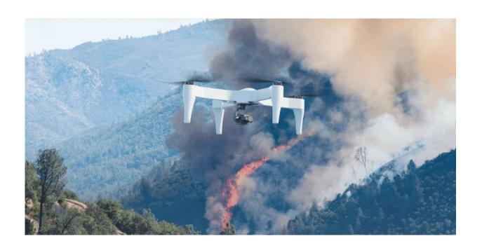
Endurance, endurance. As the drone market potential faces a hurdle in how it can respond to expectations of getting tasks done versus time in the air before needing to recharge, a newbie drone solution appears in the name of US-1 from California-based Impossible Aerospace, capable of flying 90 minutes to two hours on a single charge
