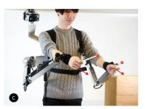
"Fusion" used as a bodily driven communication system of an operator and a surrogate. Three levels of communication are realized: (A) Direct actions using gestures and indications, (B) Enforced postures by forcing surrogate body to certain positions, and (C) Induced motions by altering the perception of body posture (red arrows represent the induced motion). Credit: *ACM SIGGRAPH* 2018 Emerging Technologies on - SIGGRAPH '18 (2018). DOI: 10.1145/3214907.3214912
