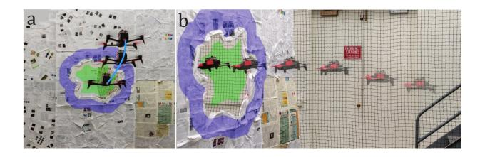
Different parts of the pipeline: (a) Detection of the unknown gap using active vision and TS2P algorithm (cyan highlight shows the path followed for obtaining multiple images for detection), (b) Sequence of quadrotor passing through the unknown gap using visual servoing based control. The blue and green highlights represent the tracked foreground and background regions respectively. Credit: arXiv:1802.05330 [cs.RO]
