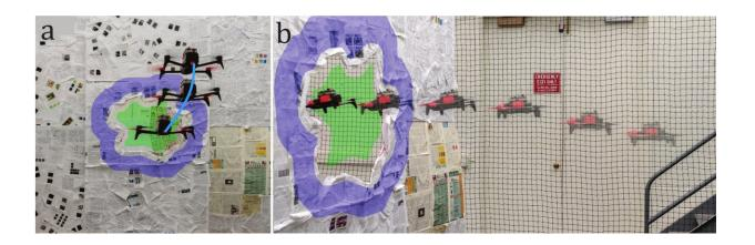
Different parts of the pipeline: (a) Detection of the unknown gap using active vision and TS2P algorithm (cyan highlight shows the path followed for obtaining multiple images for detection), (b) Sequence of quadrotor passing through the unknown gap using visual servoing based control. The blue and green highlights represent the tracked foreground and background regions respectively. Credit: arXiv:1802.05330 [cs.RO]
