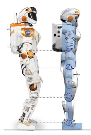
Side view of Valkyrie robot and the 2D humanoid character modelled according to Valkyrie robot. Credit: Yang, Komura & Li
