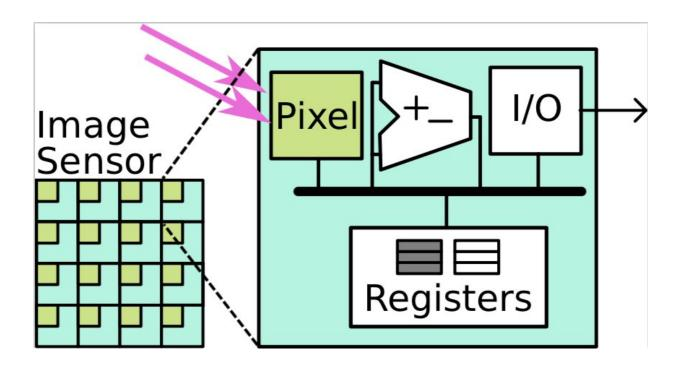
Focal-plane Sensor-Processor Arrays (FPSPs) are parallel processing systems, where each pixel has a processing element. Credit: Saeedi et al.
