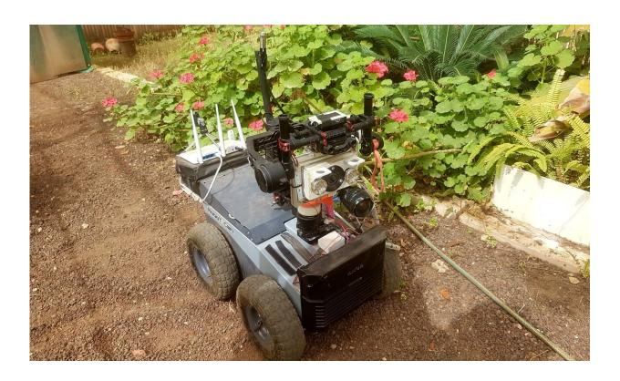
The 'Robat' -- a fully autonomous bat-like terrestrial robot that uses echolocation to navigate its environment. Credit: Eliakim et al.
