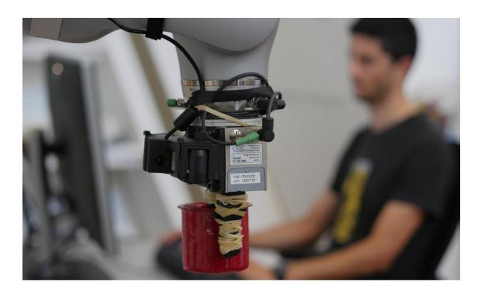
Manuelli uses the DON system and Kuka robot to grasp a cup. Credit: Tom Buehler
