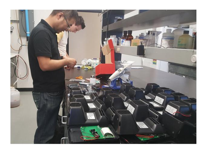
University of Utah electrical and computer engineering doctoral graduate, Kyeong T. Min, assembles air pollution sensors for a study that determines how efficient heating and air conditioning systems in the home are at cleaning the air quality while also saving energy. Credit: University of Utah
