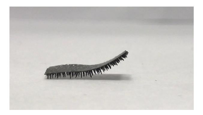
A novel tiny, soft robot with soft caterpillar-like legs which is adaptable to adverse environment and can carry heavy load was developed. Credit: City University of Hong Kong
